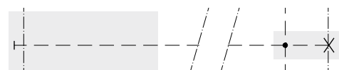
AO – Signal line open in inlet section and connected with tank in end section.
