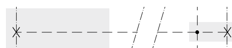
AB – Signal line plugged in inlet section and connected with tank in end section.
