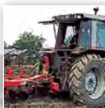
Load variation on front axle 3,5 to 100 %
